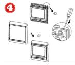
Install the housing cover and lock the external frame
